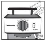
Flip open the lid of the water reservoir and the cleaning pin is located on the inside of the lid.
